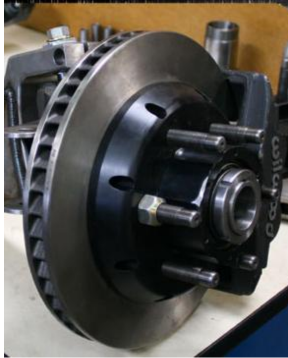
Figure 3.3.4.1 -- Rotor with cooling vanes (Brake Rotor)
